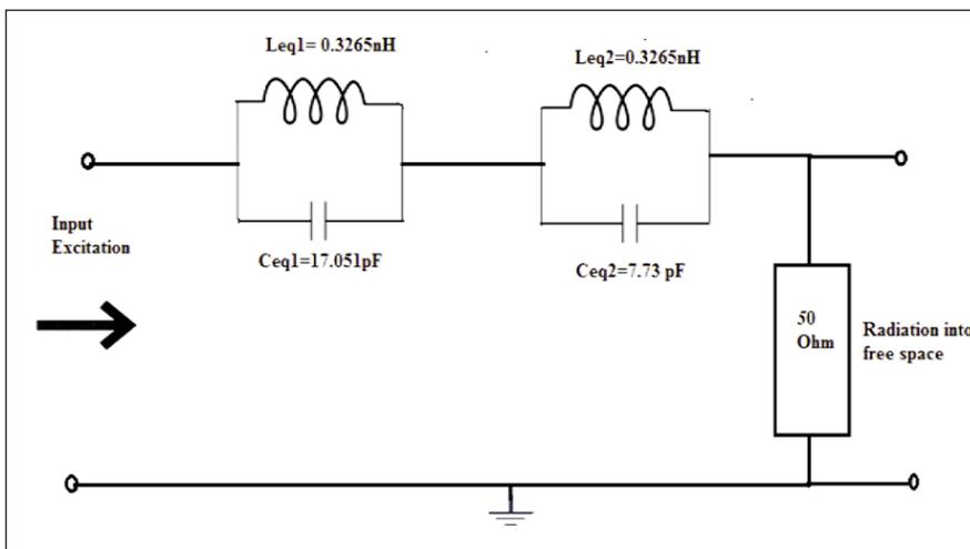
Fig. 9. Equivalent circuit model of the proposed antenna
